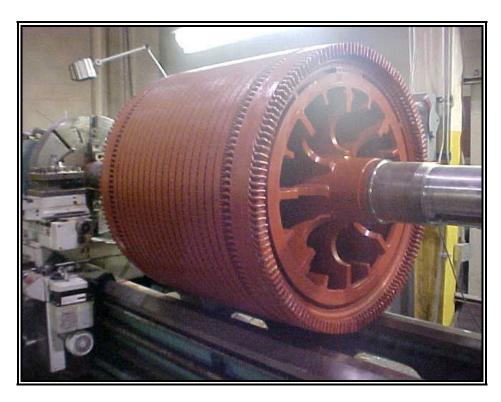
Bearing journal damaged after years of service. Plating is the best repair procedure on an assembled stator. There is <u>no heat</u> involved with this process assuring no damage to assembled unit. Using flow-thru anode, chemicals are pumped through a carbon while shaft is in rotation.
